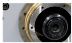
Taper hollow shafts (HSK) with flat contact faces are standardized per DIN 69893. The various shapes differ with respect to drive key slots and contact surface. Form C has been especially developed for use with manual tool change systems.
