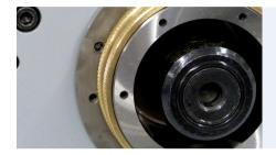
Taper hollow shafts (HSK) with flat contact faces are standardized per DIN 69893-1. The various shapes differ with respect to drive key slots and contact surface. Form C has been especially developed for use with manual tool change systems.
